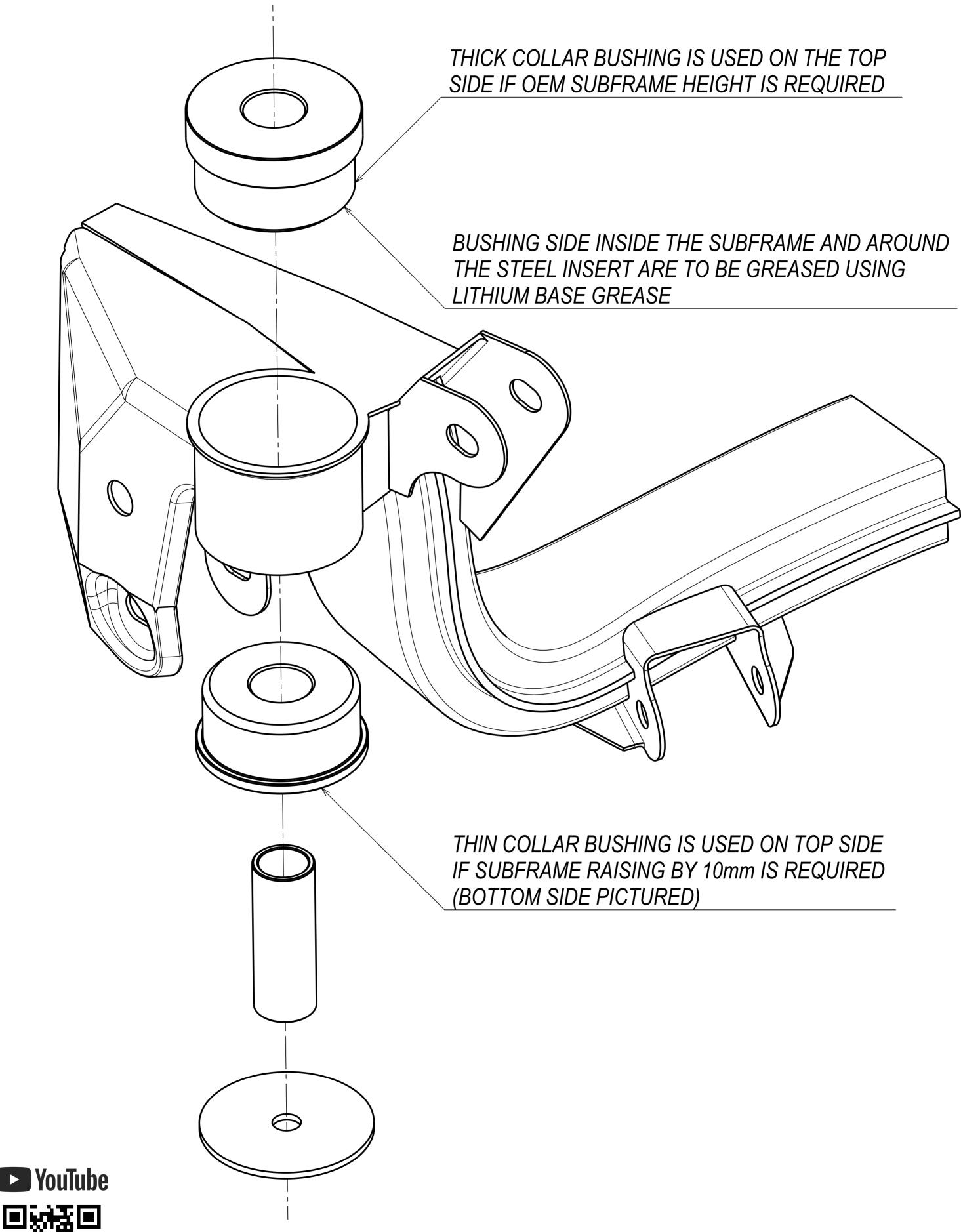
**NOTE** - The bushes are made to be an interference fit and so a press or similar may be required.
