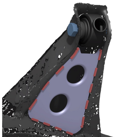
Image 11. Traction arm brace stitch welds
