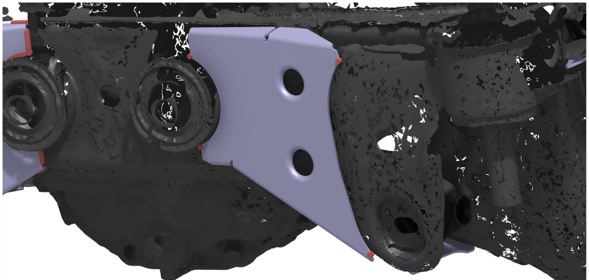
Image 5. Rear differential carrier's right side spot welding
