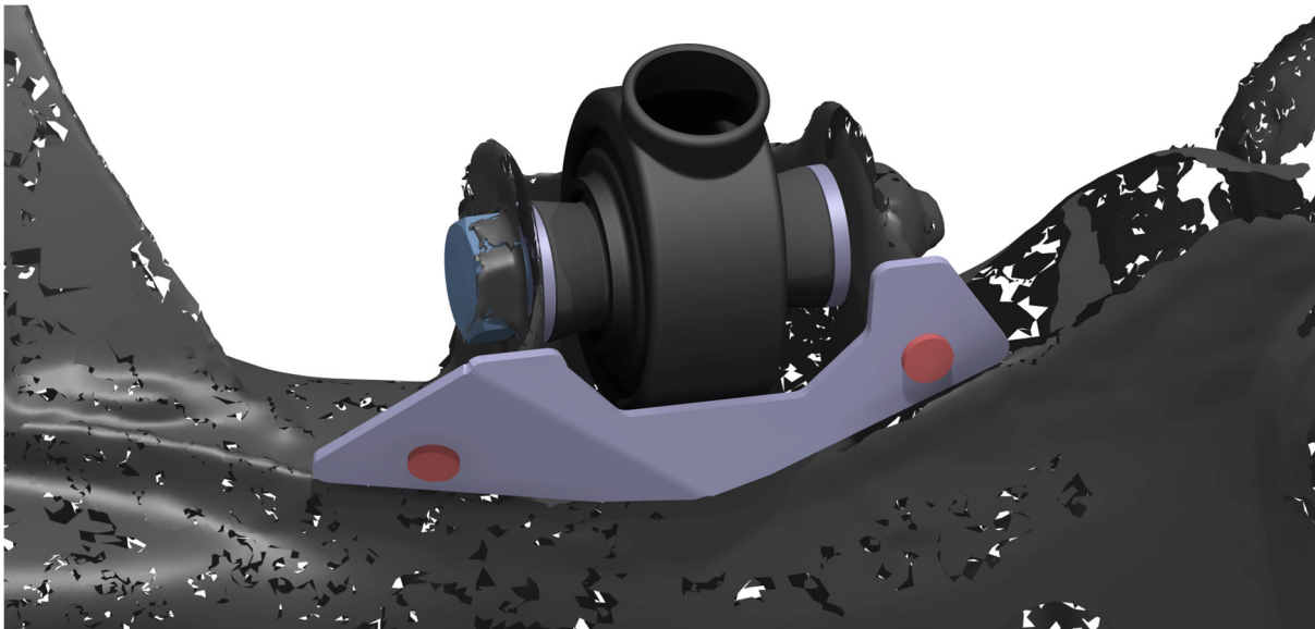
Image 15. Lower control arm front bracket brace plug welds
