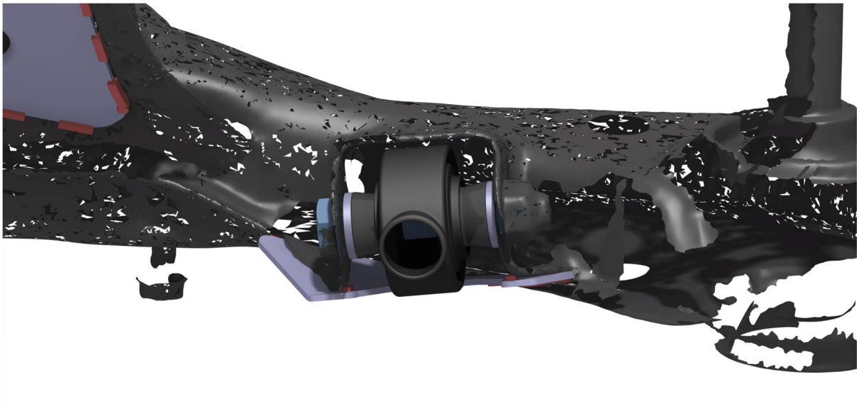
Image 17. Lower control arm front bracket brace inner stitch welds
