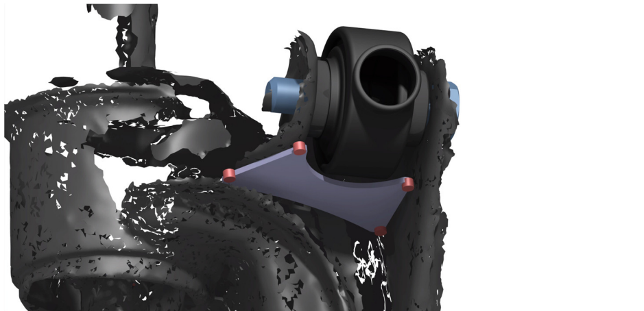
Image 8. Camber arm brace spot welds
