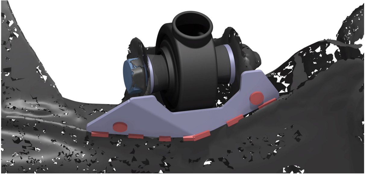
Image 16. Lower control arm front bracket brace stitch welds
