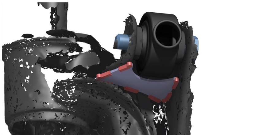
Image 9. Camber arm brace stitch welds
