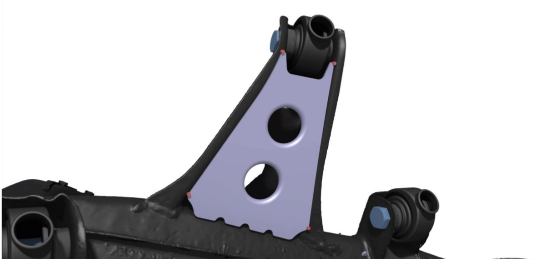
Image 5. Traction arm brace spot welds
