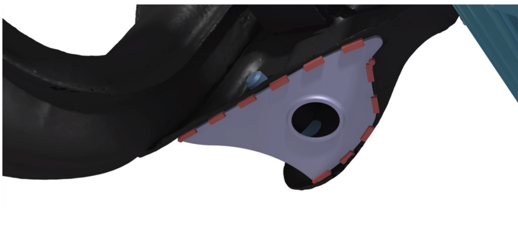
Image 14. Toe control arm bracket brace stitch welds
