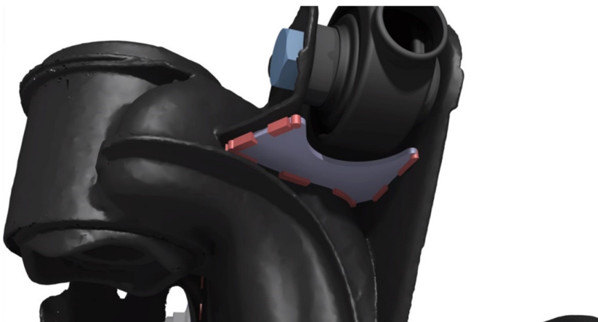
Image 4. Camber arm brace stitch welds
