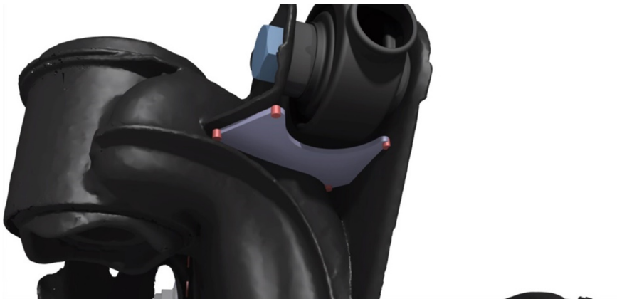
Image 3. Camber arm brace spot welds
