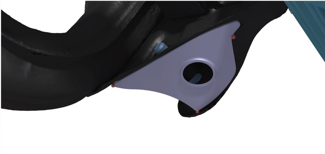
Image 13. Toe control arm bracket brace spot welds
