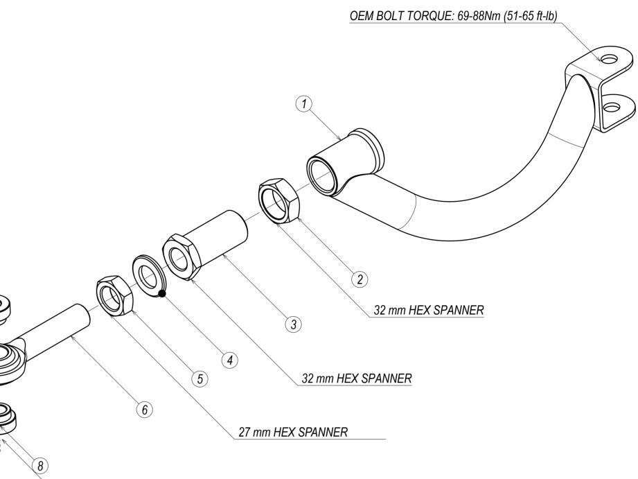
OEM BOLT TORQUE: 69-88Nm (51-65 ft-lb)
