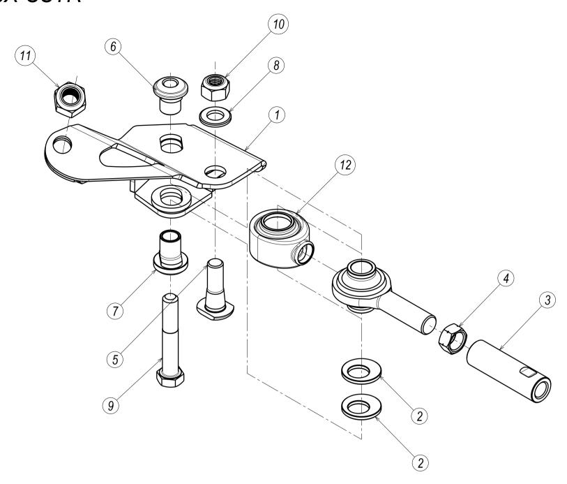
CHECK TIE ROD CLEARANCE FROM BRACKET AT MAXIMUM WHEEL DROOP (TEST ENTIRE STEERING RANGE), USE SPACERS TO INCREASE CLEARANCE,
