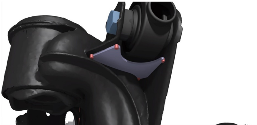
Image 3. Camber arm brace spot welds
