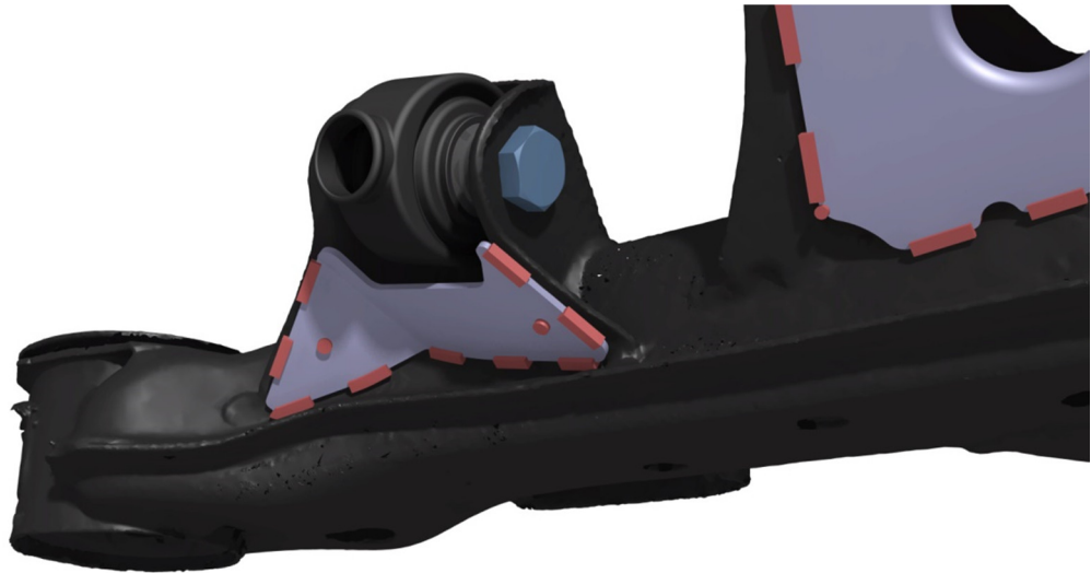
Image 11. Lower control arm front bracket brace stitch welds
