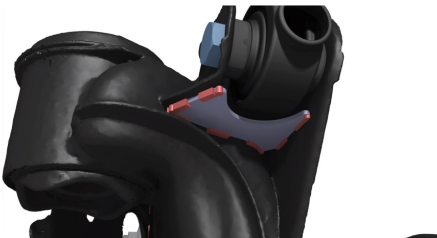
Image 4. Camber arm brace stitch welds
