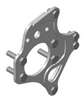
Figure 1. GKtech dual caliper bracket
